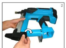
The Battery Charging and Installing
